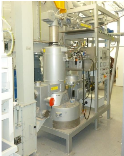
Fig. 7 Used pelleting machine KAHL 33-390
