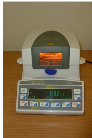
Fig. 6 Laboratory scales for measuring moisture
