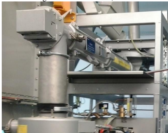
Fig. 5 Homogenizer of pelleting press with water jet
