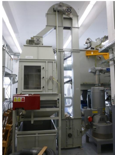
Fig. 8 Used pellet cooler with fines separation
